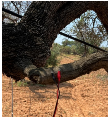
Figure 3. The electrical conductivity probes as were installed in the tree on-site.
